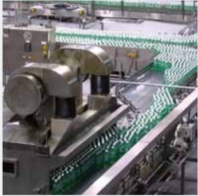
High speed buffering and pressure-less line control for bottling lines
