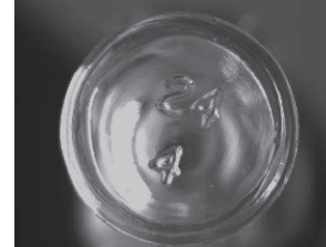
BOTTOM INSPECTION (PARTICLES AND SURFACE)
